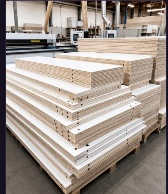
Machined panels edge-banded and staged by job for assembly
