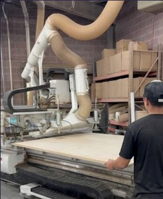
CNC nesting router — parts cut straight from the shop drawing file
