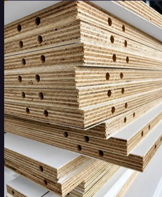
Shelf and hinge drilling referenced off a single datum
