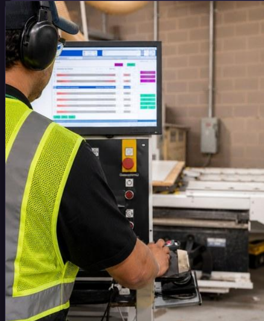
Job set-up and cut optimization at the machine control station
